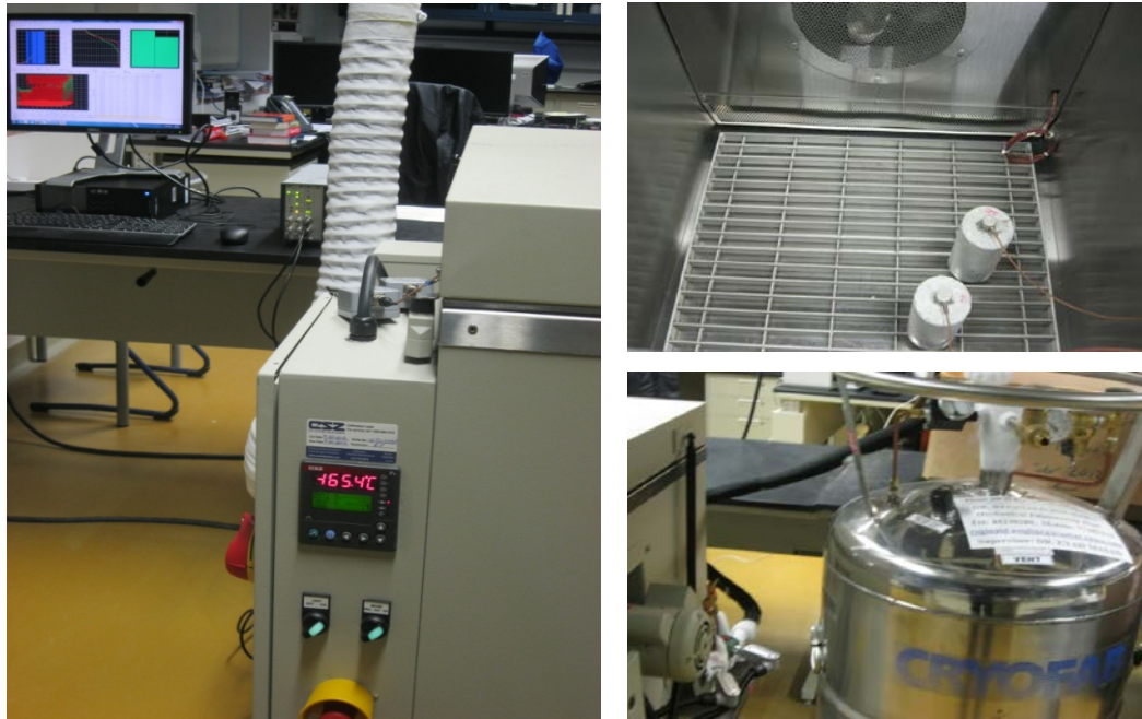
Fig. 2: Temperature chamber showing AE sensors on concrete
